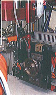
Fitting studs to a turbo- charger housing
