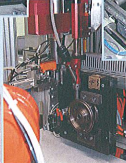
Fitting studs to a turbo-charger housing
