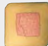
Micrograph of a square crimp
